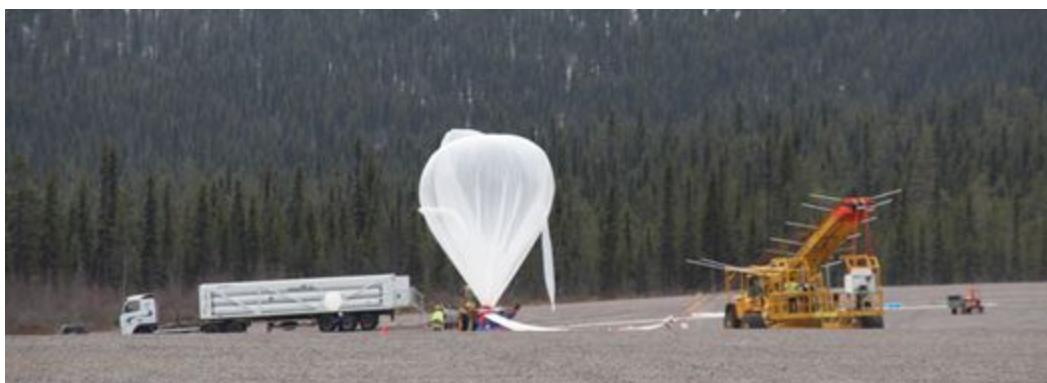
BEXUS 20 balloon shortly before take-off. The gondola with CPT-SCOPE and two other payloads is mounted in the yellow assistance vehicle called "Hercules" (right).
