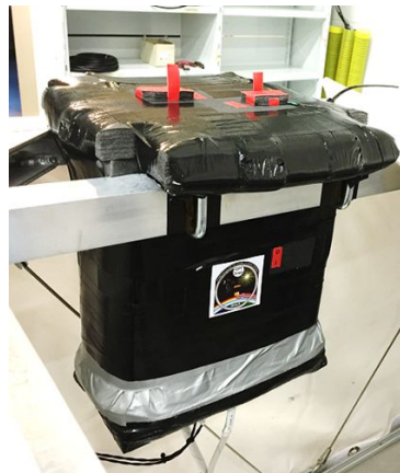
CPT-SCOPE with thermal insulation mounted inside the BEXUS 20 gondola.
